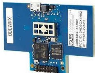
Figure 1. X4m300 UWB radar.
